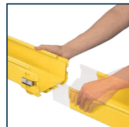
QuikLock™ Coupler provides fast connection between components without need for tools or small fasteners.
